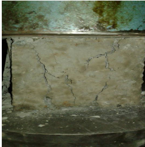
Fig 4 Testing of cube in compressive testing machine
