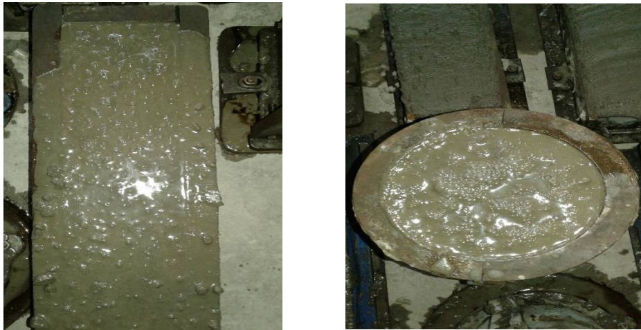
Fig 2 casting of specimens
