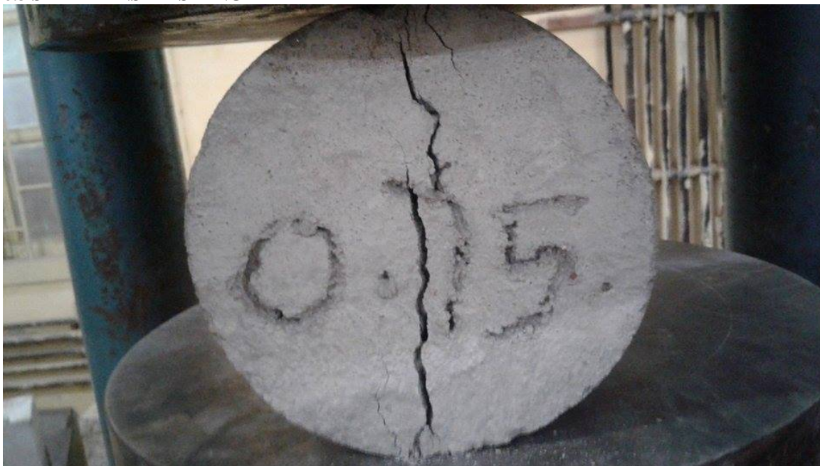
Fig 7 Testing of cylinder in compressive testing machine
